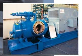
Field of Application: Chemical Process Industry/Polymer Solution Transfer Pump
